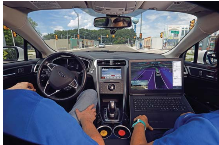
The University of Michigan's Mcity facility allows Ford to safely test our SAE Level 4-capable autonomous vehicles in a simulated urban environment. The car navigates scenarios like traffic in intersections, pedestrians in crosswalks, different traffic signals and bicyclists.
